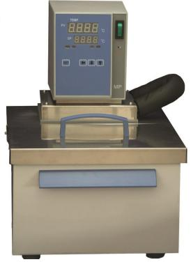
Supper Circulating Bath (Constant Temperature) Heating Circulating Bath Microprocessor Control
